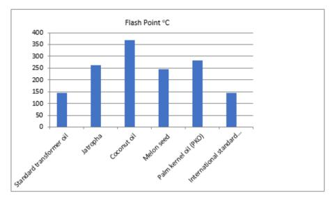
Fig. 3: Comparison between standard transformer oil and vegetable oil flash point
