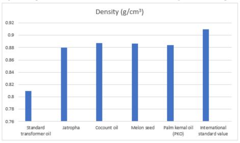
Fig. 4: Comparison between standard transformer oil and vegetable oil density
