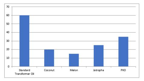
Fig. 2: Comparison between breakdown voltage (BDV) of Standard Oil and Vegetable Oils with nano-particles
